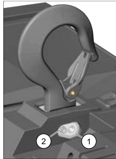
Figure 7. Suspension Pin Retainer/Retainer Screw
